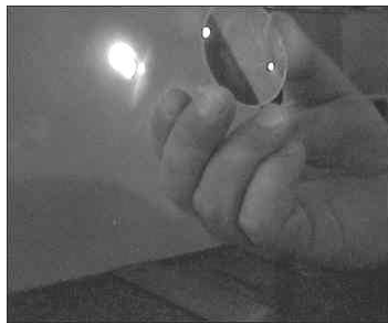
Figure 4 - Finding the focal length (20cm lens) with a ruler and light source – make the light circle as small as possible
