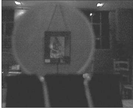
Figure 12 - The lens is close to the eye looking at a picture across the room – the erect virtual image but it will be slightly out-of-focus
