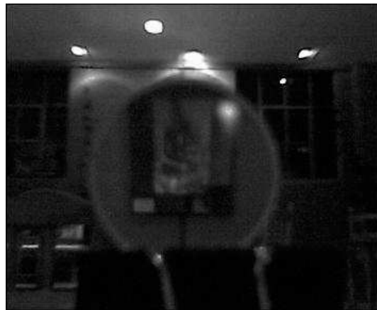
Figure 13 - As the lens moves towards one-focal length, the image of the picture on the wall remains erect and virtual but magnifies
