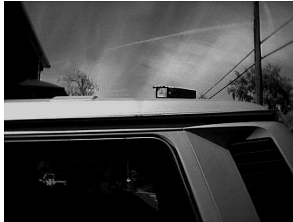
Figure 16 - Seen at about 4 focal lengths, the upside image of the telephone pole in the lens is smaller than the telephone pole itself.
